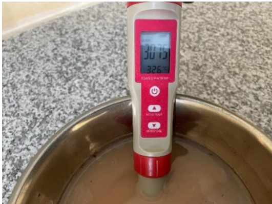
Fig-14: Checking soil salinity with EC & pH meter
