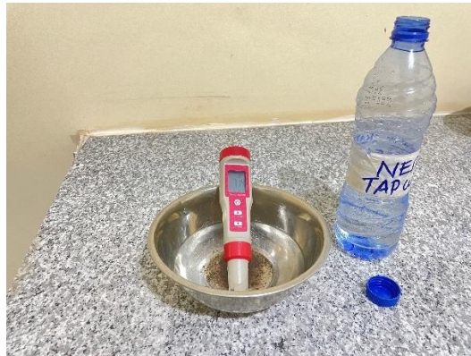
Fig-15: Checking tap water EC & pH
