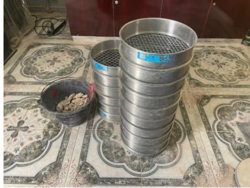
Fig-11: Sieve analysis test in progress
