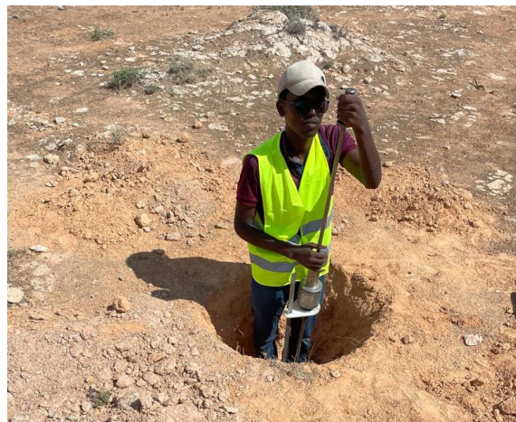
Fig-9: DCP conducted at base of a trial pit
